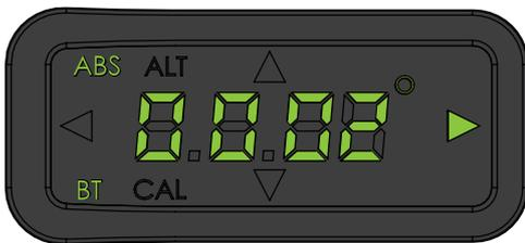
Once completed step 1 & 2, **"ABS icon"** on top left corner of display lights up to indicate that the device is in Absolute Level mode.
