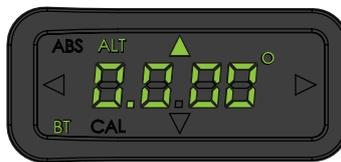
Figure 5. Device display in Alternate zero mode
